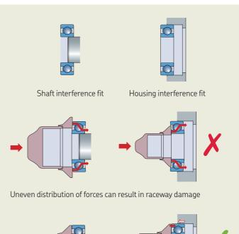
With the correct tools, raceway damage is avoided
