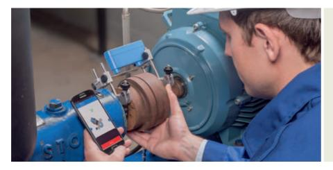
Shaft alignment is recommended for almost every industry, as it enables machine uptime to be significantly improved and maintenance costs to be reduced. The TKSA 11 focuses on industries where these shaft alignment benefits have not yet been realised and helps customers profit from correctly aligned shafts.
